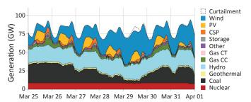
FIGURE 1. Simulated dispatch of generation over one week in a high renewable energy scenario (annual load served by 25% wind, 8% solar photovoltaic).
