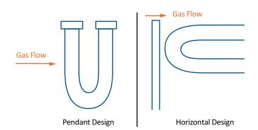
FIGURE 3. CGS has a horizontal, not pendant, boiler design, which facilitates drainage needed to reduce corrosion fatigue and allow the plant to come online faster. The pendant design more easily allows water accumulation. (Graphic: Steve Lefton, Intertek)
