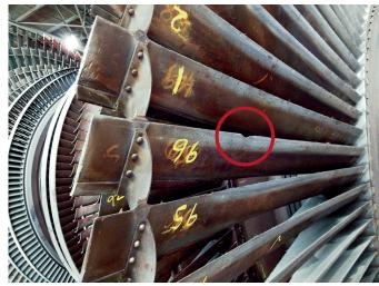
FIGURE 2. Example of large nick in turbine fin (#96) due to impact with dislodged material formed by oxidation (Debra Lew)
